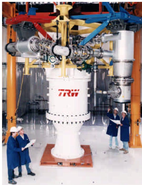
**Figure 26. The 650,000 lbf LOX/LH<sub>2</sub> Low Cost Pintle Engine (LCPE) . . . the Largest Pintle Engine Built to Date**
