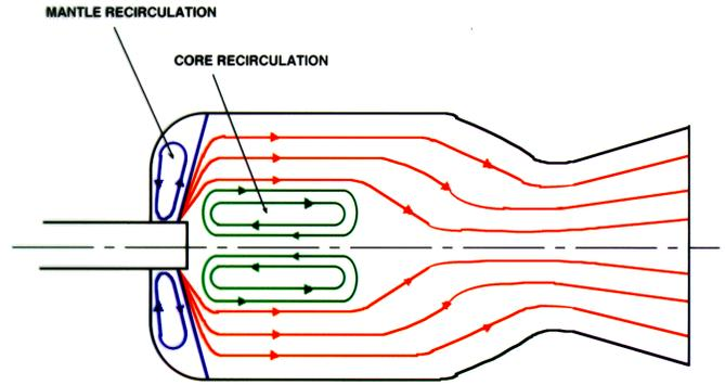
**Figure 4. Combustion Chamber Flowfield Resulting from Pintle Injection of Propellants**
