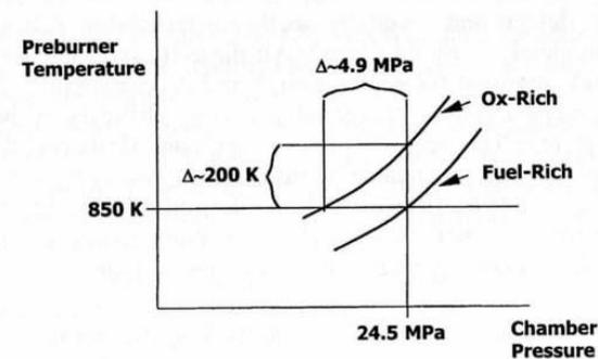
Fig. 2 Comparison of fuel-rich and oxidizer-rich turbine drive gas schemes for generation of turbine power, with 6% hydrogen propellant in engine.
