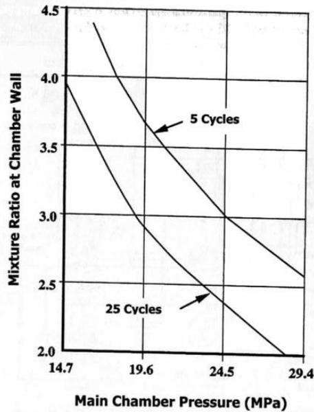
Fig. 7 Effect of number of operating cycles and main chamber pressure on the mixture ratio required at main combustion chamber wall.
