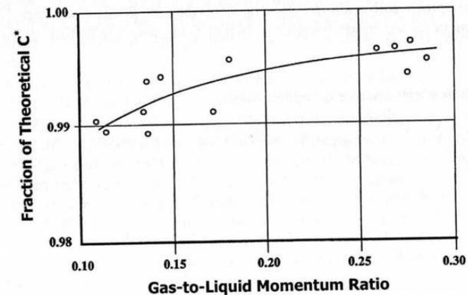
Fig. 9 Characteristic velocity efficiency of RD-0120 injection elements as function of gas-to-liquid element momentum ratio—single-element hot-fire data.
