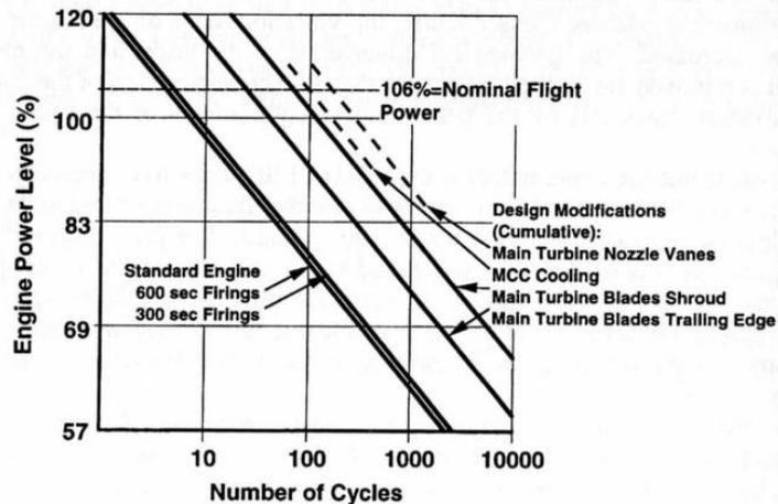
Fig. 11 Improvements in flight RD-0120 engine life due to identified engine modifications.
