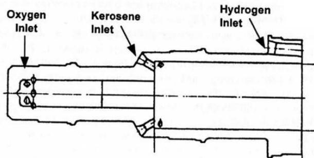
Fig. 5 Cross-section of injection element used in one-zone full-scale tripropellant preburner.
