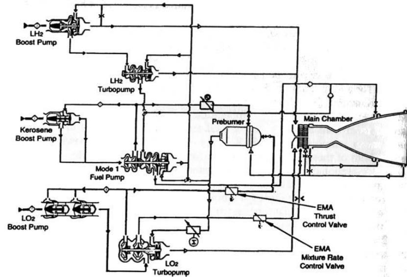
Fig. 6 Schematic of optimum closed-cycle tripropellant engine with fuel-rich turbine drive.
