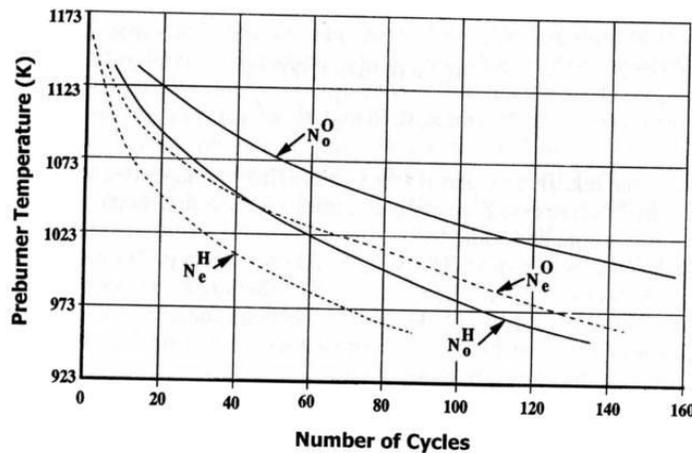
Fig. 3 Number of cycles to crack initiation ( $N_o$ ) and operational cycles ( $N_e$ ) as functions of preburner gas temperature and fuel-rich (H) and oxidizer-rich (O) turbine drive gas.
