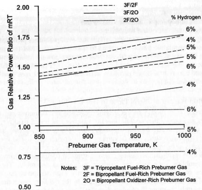
Fig. 1 Comparison of relative turbine drive gas power capability.
