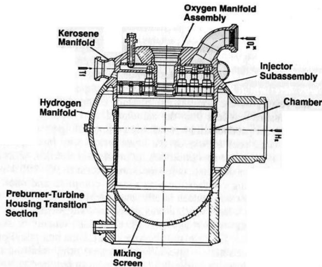
Fig. 4 Cross-section of one-zone full-scale tripropellant preburner.
