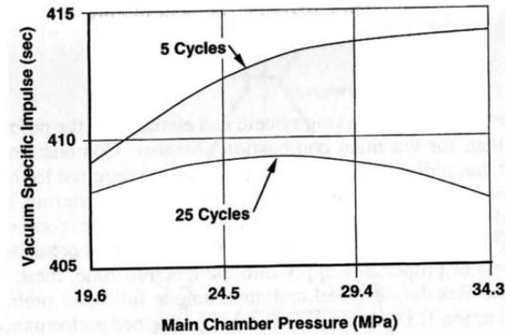
Fig. 8 Effect of main chamber pressure and number of operational cycles on vacuum specific impulse.
