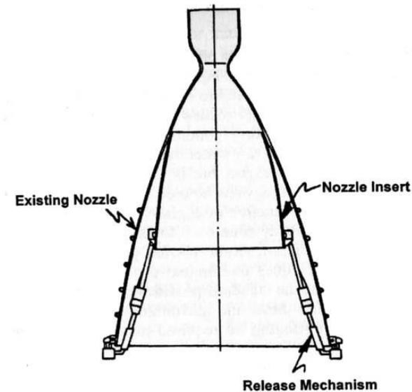
Fig. 10 Altitude compensating nozzle insert for tripropellant engine with single bell nozzle.
