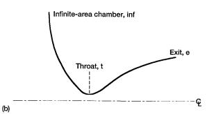
Figure 6.1.—Schematics of rocket combustion chamber cross sections. (a) Finite-area combustion chamber. (b) Infinite-area combustion chamber.
